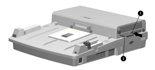
Figure 7-7. Removing a PC Card
